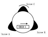
(3) Turn around the instrument 90° again. Repeat above steps until the bubble remains in the center of the plate level even though the instrument is rotated to any position.
