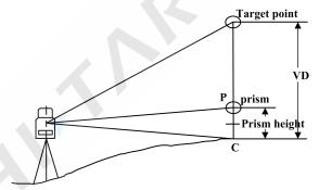
There are two modes for 'REM' measurement: 'Input TH' and 'without TH'. You can select 'Input TH' mode when you need the altitude from ground to target, otherwise 'without TH' when you need the altitude from any reference point to target.
