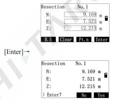
5) Press [F4](Yes) to enter the interface of "Input T.H". After input the target height (T.H), press [F4];
