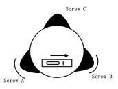
(2) Turn the instrument approximately 90° and adjust screw C until the bubble in the center of the level;
