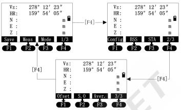
• Save:After press [F1], the interface of "Information" appears (if you haven't select measured file, there will be a interface of "Select file (.MEA)" to let you select file.), which needs you the point name (Pt.N) ,Code and target height (T.H). The number of "Pt.N" defaults to added 1. The code is input according to your need, but the target height according to actual situation. You can press [ENT] to save data to measured file.
