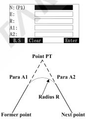
'PT' is the intersection point of road. The "x" of "Px" is the number of intersection point.
