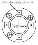
Note: Check the photoelectric coaxiality after calibrating.
