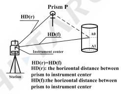
When measuring the coordinate of the earth point'A1' which is the projection of 'AO', set up the height of instrument and the height of target.
