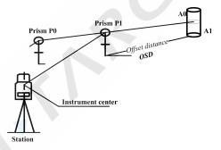
Firstly, input the offset distance. If the directions of "P1-A0" and "P0-P1" are same, the distance value is positive, otherwise it is negative.
