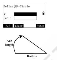
The value of Radius (R) can be negative. The positive direction is the right direction along the designed roadway, and the left is negative. The "Len." refers to Arc length.
