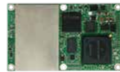
Advanced BD970 OEM is a compact multi-constellation receiver designed to deliver centimeter accuracy to a variety of applications.
